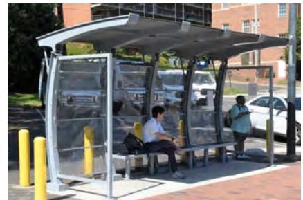
foot deep roof supported by strong curved "I" beam columns and escutcheon covered base plates. Full-length wind-protecting end walls and full height rear walls are made of durable aluminum frames with clear polycarbonate panels that provide both high visibility for passenger security and clear sight lines for approaching bus operators, while enhancing passenger comfort by providing protection from wind and rain.
